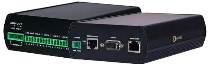
The AMP523 is a Mini Stereo Amplifier with an Integrated web based control unit, featuring four stereo line inputs and one balanced microphone input with phantom power. It has an output power rating of 2 x 15 Watt.
