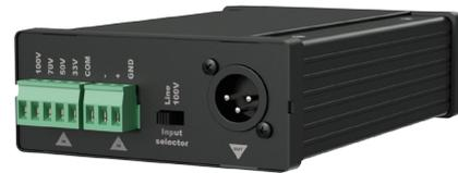
The ATU44MK2 is a universal input adapter unit for conversion between various audio level signals, offering a wide variety of connection and extension possibilities to audio systems. The speaker level input features various tapings for 100V, 70V, 50V and 33V audio levels, while a balanced line input allows conversion between balanced and/or unbalanced line level audio signals.
