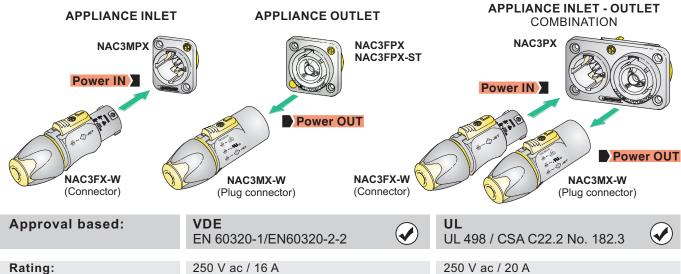
Rating: 250 V ac / 16 A Cable Type: H05VV-F3G 1.0 mm², Length max. 2 m H05VV-F3G 1.5 - 2.5 mm<sup>2</sup> H07RN-F3G 1.5 mm<sup>2</sup> Strain Relief: White chuck Cable O.D.: 6.0 - 12.0 mm
